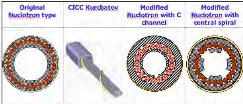
Figure 4. Cable design options for increased cooling and energy margin that are being considered for the SIS100 dipole magnet. A short cable test is planned to compare the performances of selected designs
