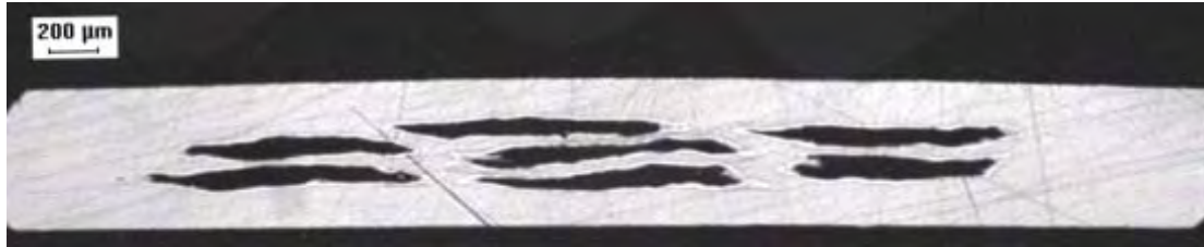
Fig. 6: Transverse cross section of a multifilamentary tape with similar critical current than the monocoresh. A diffusion barrier in Niobium is present around each filament.
