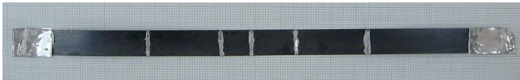
Fig. 7. A strip of the Bi-2212 coated tape , with voltage taps for transport V(I) measurement
