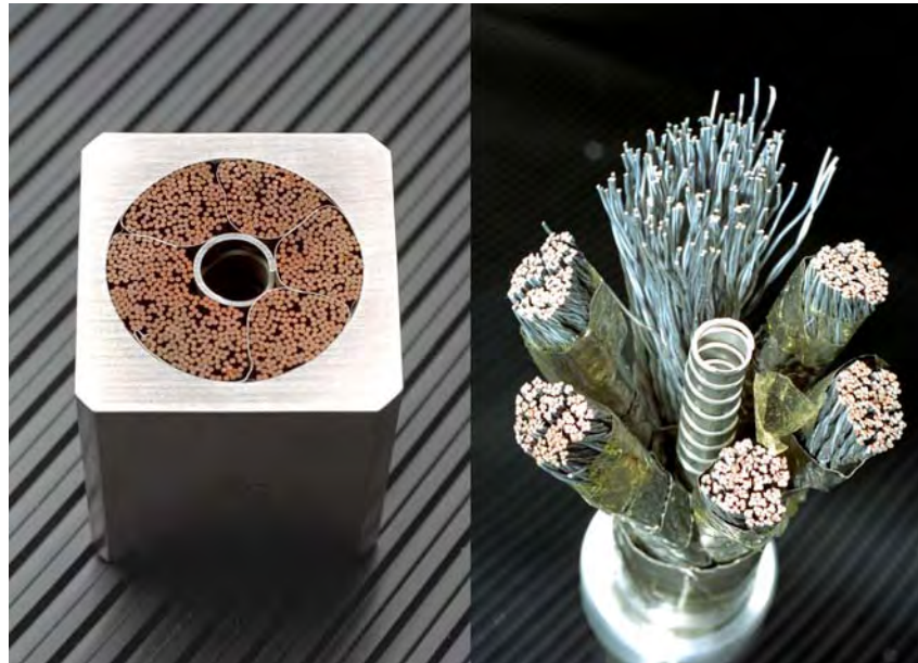
Fig. 10: picture of a section of the full-size Cable-in-Conduit Conductor adopted for the ITER magnets. External jacket dimensions are about 50 mm x 50 mm.
