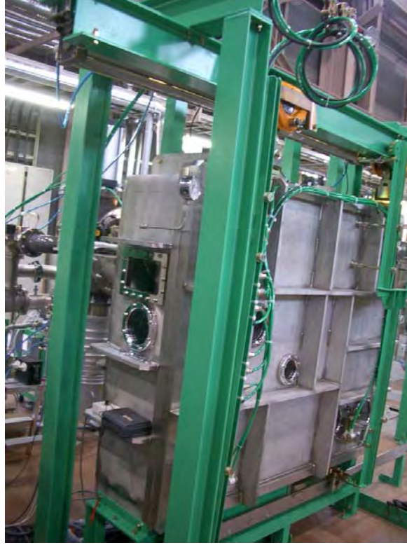
Fig. 4 A newly installed reel-to-reel joule heating apparatus at the NIMS, which is designed to process a long-length of RHQ operation over 2 km for a wire 1.35 mm in diameter.
