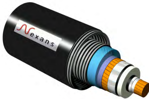
Fig. 2 - Cold dielectric superconducting cable. This is a coaxial cable where the dielectric between core and shield is maintained at cryogenic temperature.
