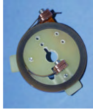
1 st pancake winding from 10m YBCO CC
