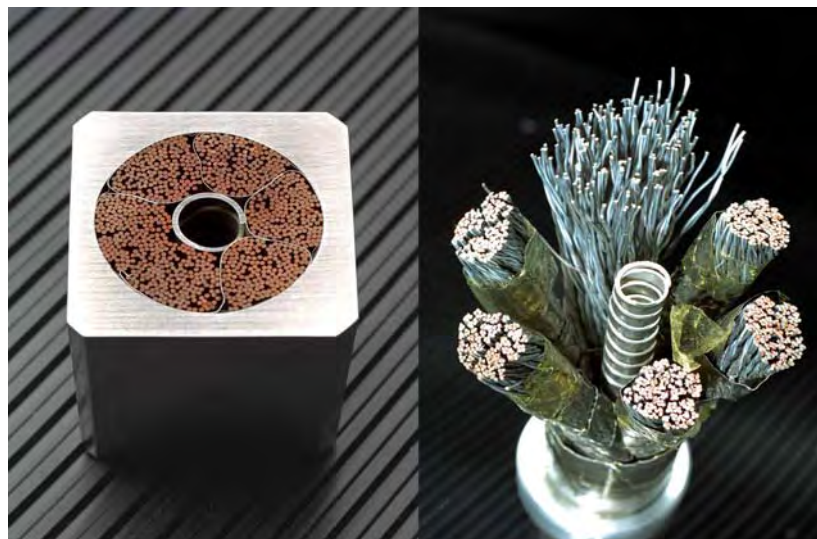
Figure 3. Conductors of the two ITER model coils: CSMC conductor, left, exploded TFMC conductor, right.
