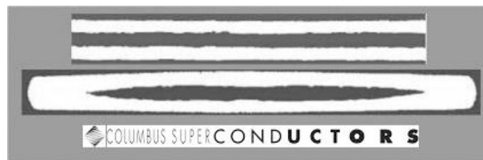
Fig.4. Cross and longitudinal section of a monocoil tape produced by Columbus Superconductors
