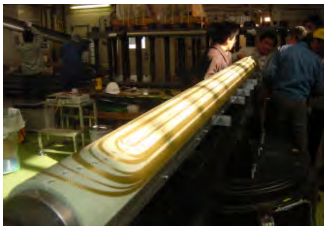
Fig. 5 Test winding at KEK of the left/right asymmetric coil for the combined function magnet for the J-PARC neutrino experiment.
