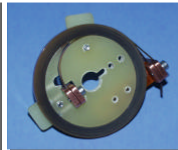
1 st pancake winding from 10m YBCO CC
