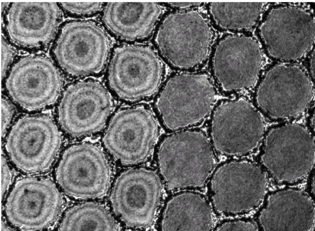
**Figure B3.3.8.** This billet was inadvertently stacked with Nb-Ti rods from two different raw material sources. On the left, the characteristic “tree ring” pattern indicates that these rods were not properly remelted, and have variations in local chemistry due to the large separation between the liquidus and the solidus. On the right, much more uniform chemistry is indicated by the uniform contrast of the Nb-Ti rods.
