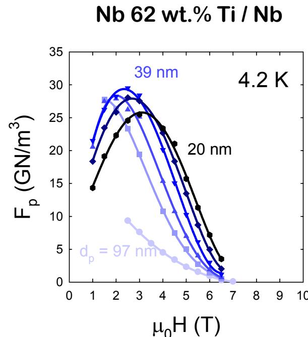
Nb47Ti/Nb APC is too Nb-rich, while Nb62Ti/Nb APC should be about Nb47Ti
