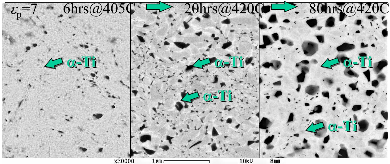
$\alpha\text{-Ti}$  precipitates are dark in backscatter SEM images, Nb-rich are light
