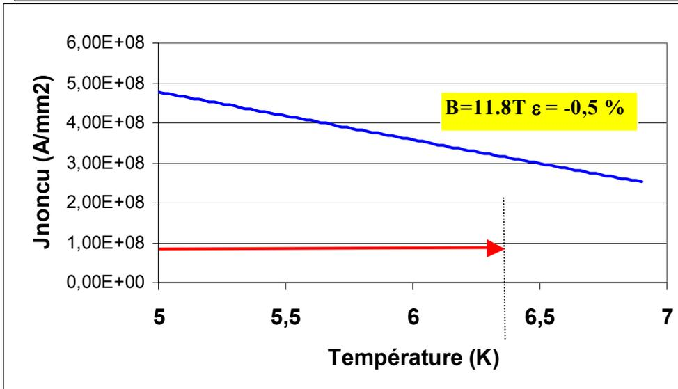
**0.2 % in addition in compression is equivalent to 1.3 K temperature increase In ITER TF conditions**
