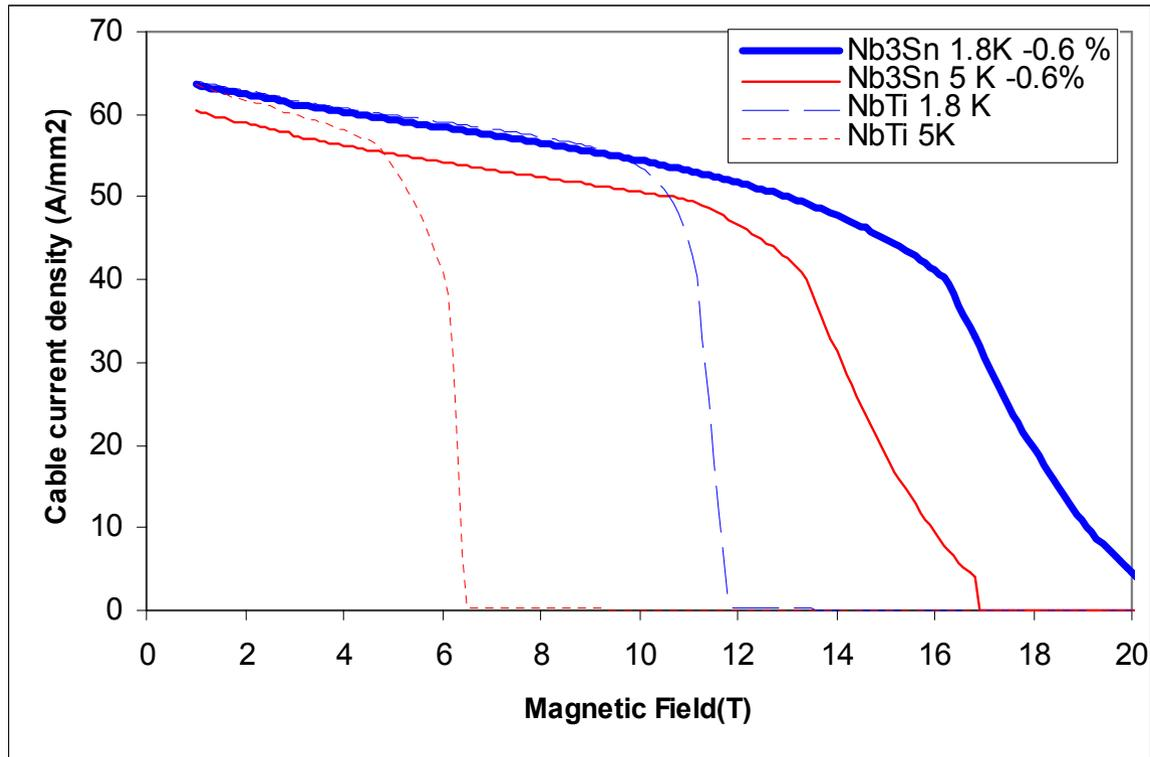
Range of application of NbTi and Nb<sub>3</sub>Sn as a function of field and temperature
