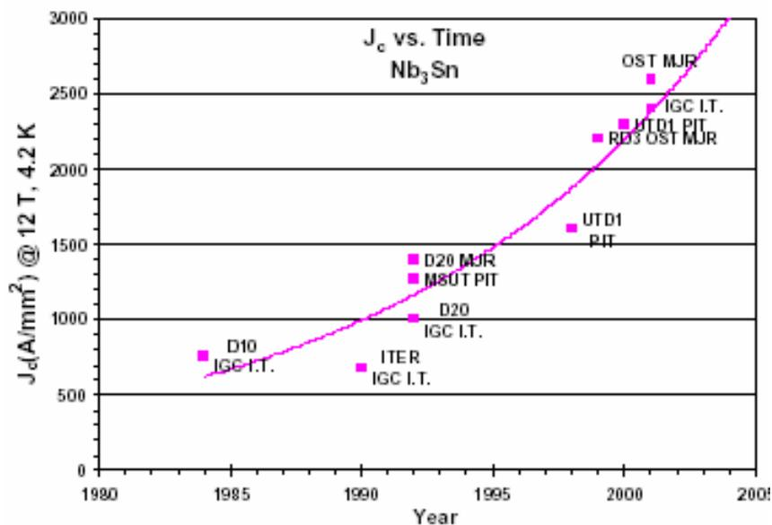
Figure 8.R4.4.3: Improvements of  $J_c$  (12 T, 4.2 K) of Nb<sub>3</sub>Sn wires since 1984 (from Fermilab Report TD-01-01, 14 Feb 2001).
