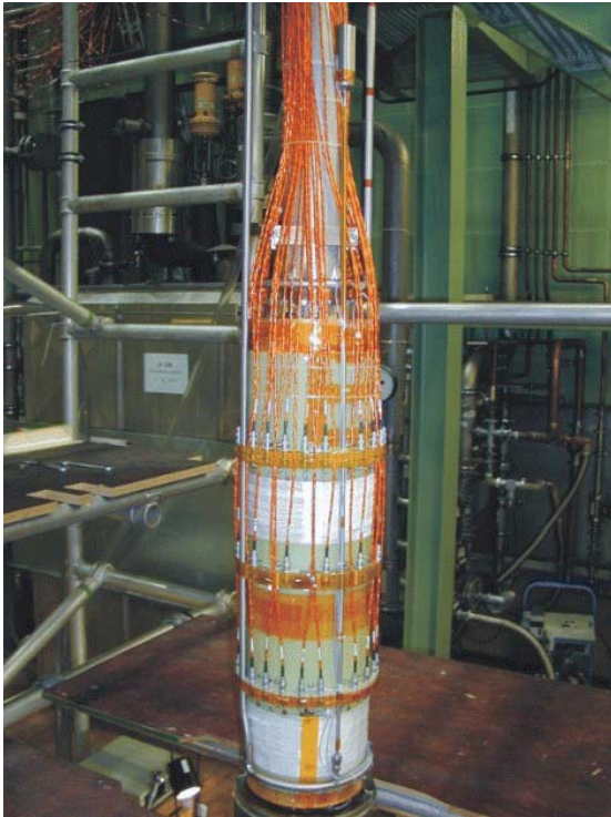
HTS-module with instrumentation cables
