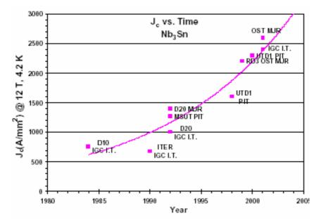
Figure 8.R4.4.3: Improvements of  $J_C$  (12 T, 4.2 K) of Nb<sub>3</sub>Sn wires since 1984 (from Fermilab Report TD-01-01, 14 Feb 2001).
